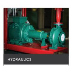
End-suction back pull out (as required by the EN 12845 - 10.1 standard) horizontal axis standardised centrifugal pump coupled with an electric or Diesel motor by means of an elastic spacer coupling protected by safety coupling cover.
